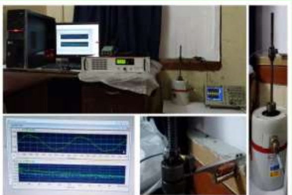
Experimental Setup of the Magnetostrictive Energy Harvester using Shaker and other accessories
